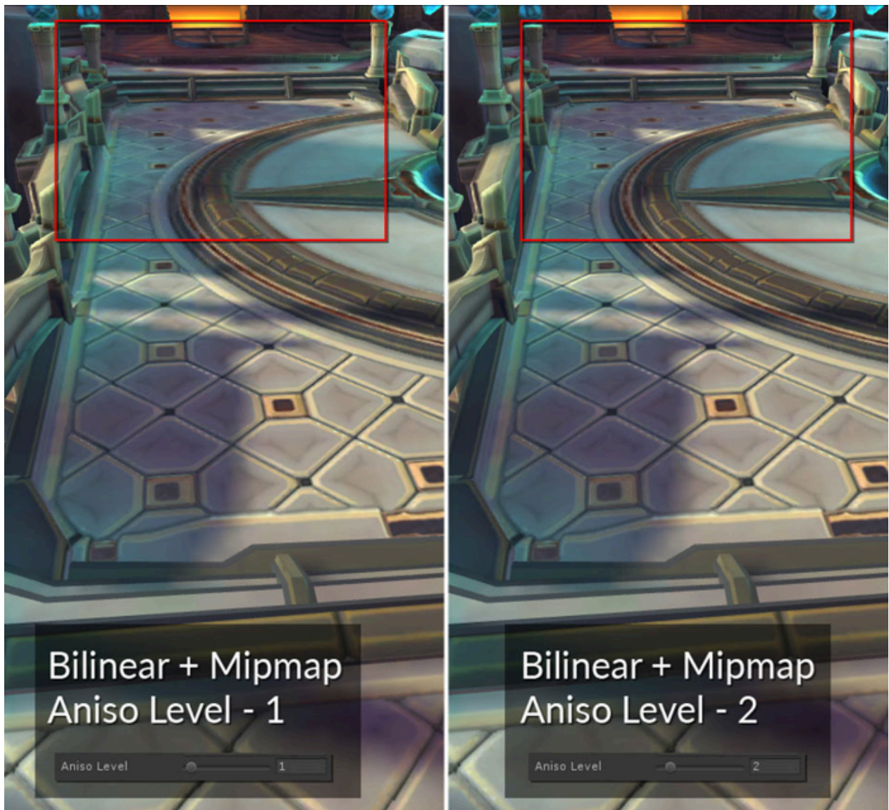
Figure 3-3: Anisotropic filtering
